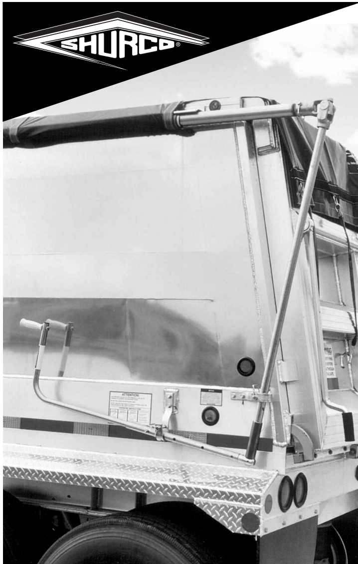
Above: The exclusive Shur-Flex™ crank arm shown on an end dump.
