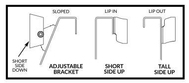
Above: Position single bow brackets according to the width of the rails, with short side up for lip in boxes and tall side up for lip out boxes. If using the Adjustable Bow Bracket for carts with sloped side rails, position the short side down.
