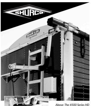
Above: The 4500 Series HD has been designed with spiral spring returns, front and back, a flexible elbow and heavy-duty front and rear torsion arms. Its Americanmade motor has an allmetal casing and a superreliable magnetic brake.
