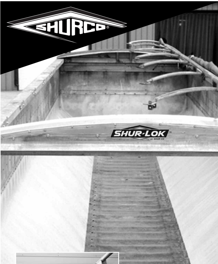
Above: The Electric Turning Point™ Bow System moves bows out of the way while you remain safely in the cab. Left: The electronic actuator.
