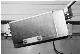
Above: The Electric Turning Point™ Bow System moves bows out of the way while you remain safely in the cab. Left: The electronic actuator.
