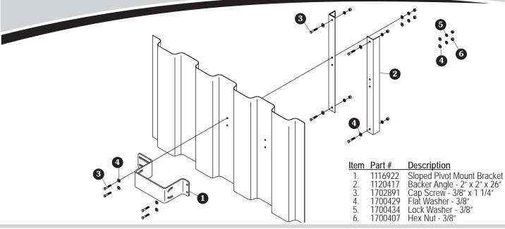
STEP 1: Determine pivot mount bracket locations according to instructions for sloped trailers in 4500 Owner's Manual.
