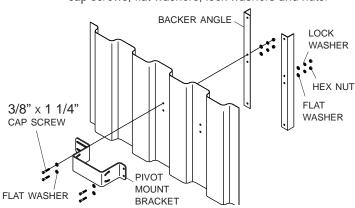
STEP 5: Using remaining holes in backer angles as a guide, drill holes in trailer. Fasten angles to trailer with 3/8" x 1" self-tapping screws, flat washers, lock washer and nuts.
