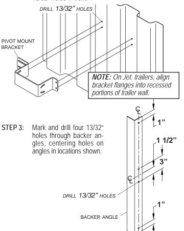
STEP 4: Place backer angles inside kingpin, aligning flanges as shown. Place pivot mount bracket on front of trailer and align holes in bracket and angles with holes in trailer. Fasten angles and bracket to trailer with 3/8" x 1 1/4" cap screws, flat washers, lock washers and nuts.
