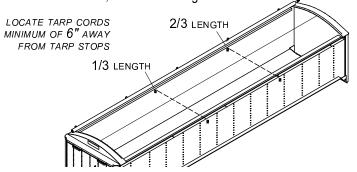
STEP 2: On tarp stop side of trailer, determine vertical rows of rivets nearest to marks below top rail. Drill hole between two rivets, just below trailer frame.
