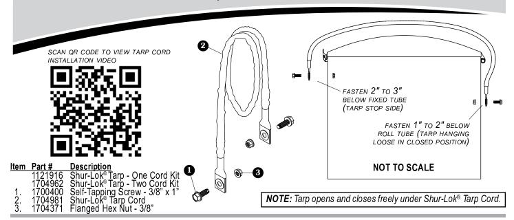
**NOTE:** Where 3/8" x 1" self-tapping screws **①** are used, use nuts on interior side, if possible, and drill 13/32" holes. If interior side of trailer is not accessible, self-tapping screws used without nuts require minimum wall thickness of 3/16". Drill 5/16" holes.
