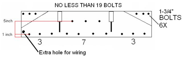
Note: 8 (1-3/4"), and 15 (3-1/2") bolts supplied. Adjust this pattern to suite the individual trailer. Account for airlines, beams, wiring, and any other variables.
