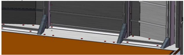
d) Drill at least two (2) 9/16"-diameter holes into each 3"x3" angle piece (within ~2" from each post if possible) and bolt in 1/2"-diameter bolts. Drill at least four (4) holes through the base plate and/or a 3"x3" angle approximately 1/4" tangent to the outside of the trailers support I-beam.
