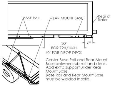
4. The Base plate will sit on top of the rub rail and flush with the deck, 6" from the rear of the trailer as shown in **Picture 1**.
