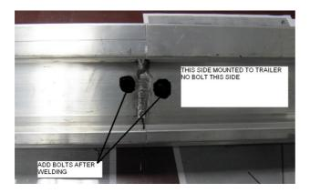
Note: Both ends must align exactly or you may have problems inserting the track insert.
