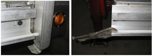
Note: If the headboard is not installed, secure at the front with a pair of vice grips. Do not proceed to the next step until the headboard, and the wings (side frames) have been installed.
