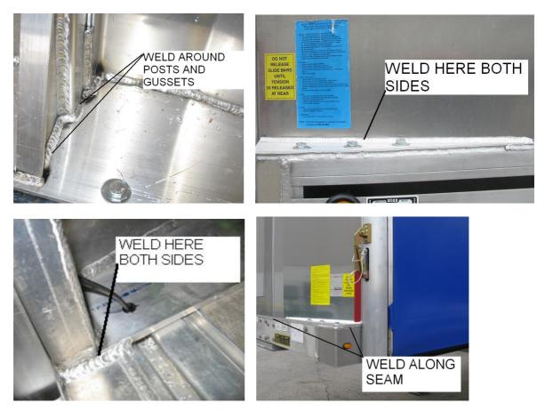
2. For aluminium trailers weld along the seam between the front of the trailer and the headboard mount plate. Grooving may be required to allow for better penetration of the weld.
