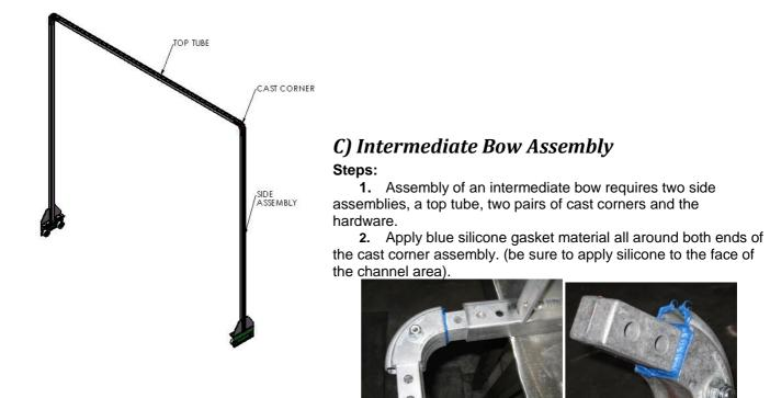
3. With a pair of corners sealed, install in the tubes and fasten with the hardware provided.
