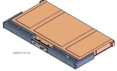
8. Drill holes and install the Corner Angle Support (RTC-01313)
