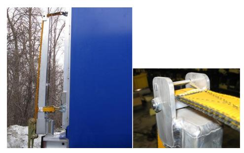
Note: the rod must be to the outside of the system away from the rear flap area
