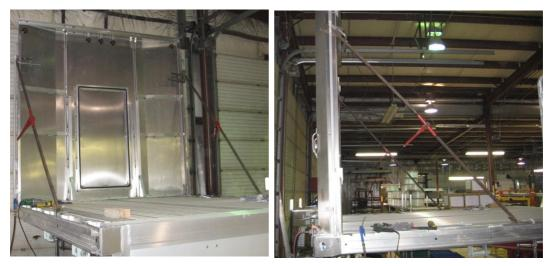
**Note:** Add shims to fill gap under Headboard at bolt locations. Too much gap under the headboard and it might bow at the top when bolts are installed.
