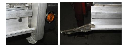
6. From underneath the track Drill a  $\emptyset$  9/32 hole up through the center of the nylon insert and insert a 1/4" flat head screw down through the hole and fasten with a nut so the screw head is flush with the insert.
