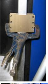
7. Clamp the Two Lifter Brackets (at the bottom end) to the bow using the C-jaw vice-grip and measure the distance from the bow foot on both sides. See how the lifters sit on the tarps. Re-adjust and repeat if necessary.
