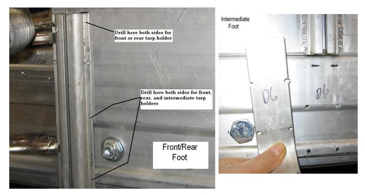
8. Label the location for each holder and the foot it belongs to. The picture below shows the holder belongs on the sixth intermediate bow (53' system) on the driver's side.
