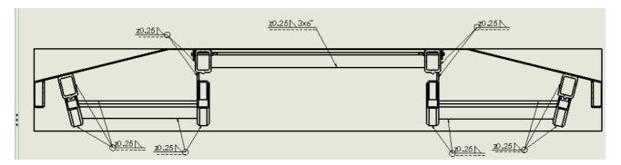
j) Drill at least two (2) 9/16"-diameter holes into each 3"x3" angle piece (within ~2" from each post if possible) and bolt in 1/2"-diameter bolt.
