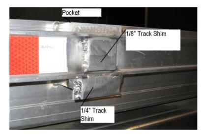
3. Mark the deck at the center of the stake pockets to locate the shims for **Track Installation** (page 12)
