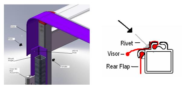
**3.** Install three rivets RTC-15071 with large steel washer RTC-14123 and rubber washer RTC-16014 evenly spaced from the corners and one in the middle.
