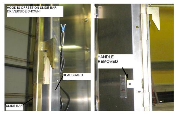
3 Slide the appropriate side frame (wing) onto the slide locks making sure to slide the bottom handle mount through the tarp seal on the inside of the side frame and out through the slot.
