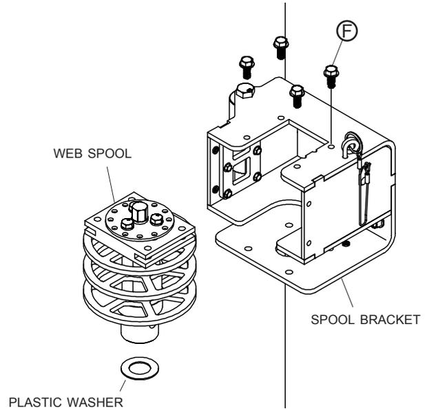
**STEP 7:** Insert motor shaft through plastic washer and hole in spool bracket. Secure with four 5/16" flanged lock nuts **Q**.
