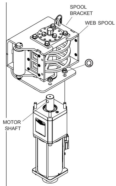
**STEP 8:** Rotate web spool so M8 x 120 screw is facing forward. Remove screw and loosen other two screws so two bushing spacers can be removed.
