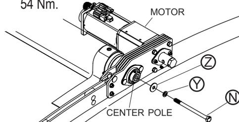
**STEP 5:** To adjust pivot arm and drive/motor assembly to be in contact with hood, rotate cams upward until tight. Tighten all fasteners securely.
