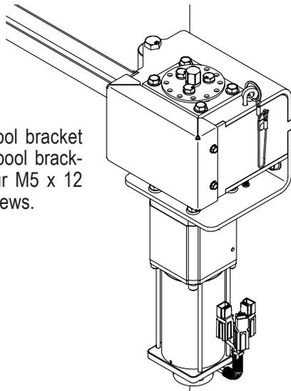
**STEP 6:** Reconnect white quick-disconnect for spool motor wire. Press and hold close button. Allow webbing to roll up on spool until 2430mm mark reaches bracket. Two people may be needed to safely complete this step.
