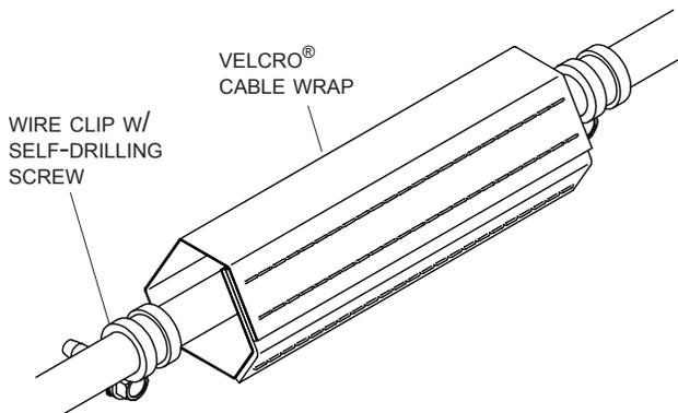
**STEP 6:** Route connected wires from spool motor to wireless receiver. Secure wire to bottom of spool bracket with 5/8" wire clip and screw **(B)**. Secure to gear box with 1/2" wire clip and screw **(B)**. Secure wire to trailer with 5/8" wire clips and self-drilling screws **(B)**.
