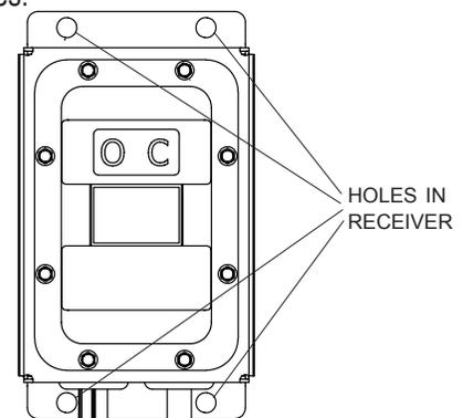
**STEP 3:** Align holes on wireless receiver with holes on trailer. Fasten with screws **(H)**, washers **(X)** and nuts **(R)**.
