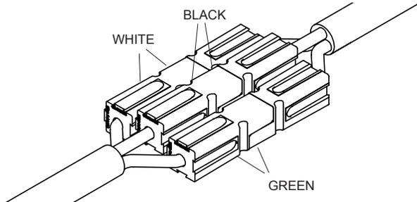
**STEP 17:** Cut Velcro® cable wrap into six 6" pieces. Wrap around wire connections. Secure wire with wire clips.
