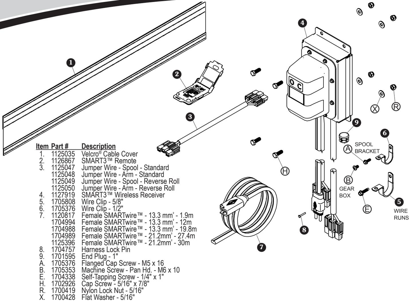
Follow these steps if wiring wireless receiver onto front skin of trailer. Skip to step 10 if wiring behind skin of trailer.
