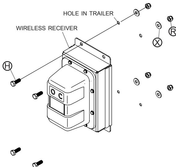
**STEP 15:** Drill hole in location shown and install rubber grommet with 14mm ID (grommet not supplied).
