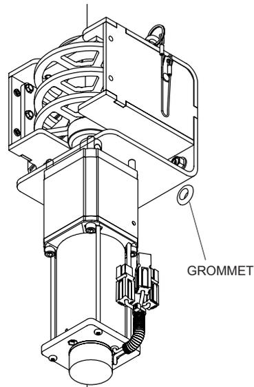
**STEP 16:** Connect jumper wire between wireless receiver wire mandrel spool and wire connected to spool motor. Connect wire ends to matching colored wire ends.
