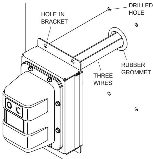
**STEP 14:** Align holes on wireless receiver with holes on trailer. Fasten receiver to trailer with screws **H**, washers **X** and nuts **R**.
