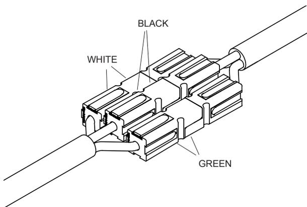
**STEP 5:** Cut Velcro® cable wrap into six 6" pieces. Wrap around wire connections. Secure wire with wire clips.
