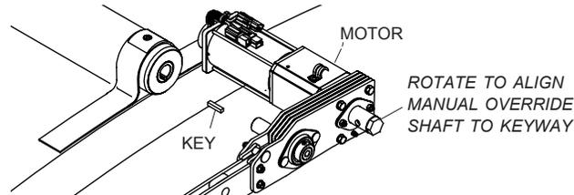
**STEP 4:** Secure drive motor to center pole with fender washer Z, lock washer Y and cap screw N. Torque bolt to 54 Nm.
