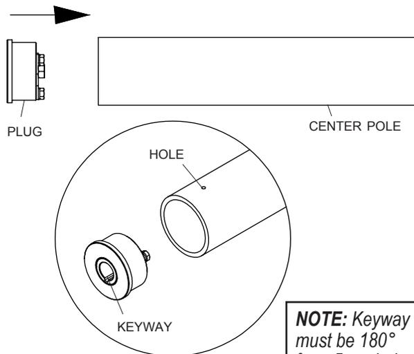
**STEP 6:** Weld center pole plug assembly onto end of center pole.
