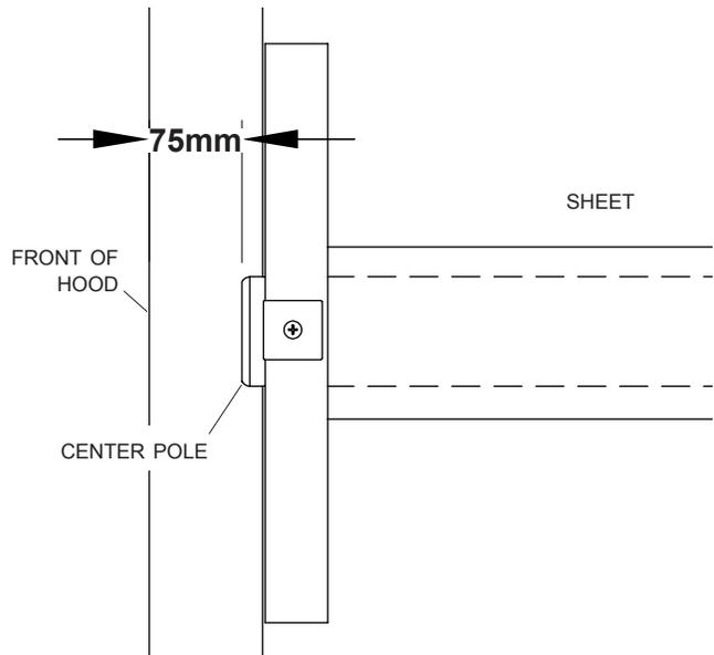
**STEP 11:** Secure fixing bar to box using preferred method. If using sheet stops, mount first and last sheet stops 320mm from edge of sheet. Equally space remaining sheet stops.
