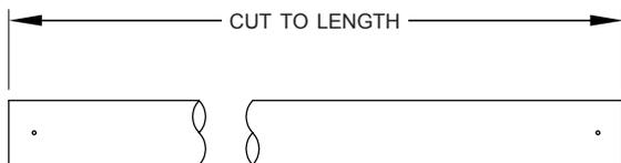
**STEP 4:** Verify ends of center pole are cut at 90°.
