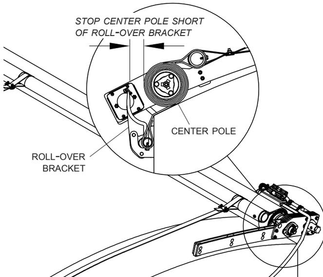
**STEP 10:** Unplug white quick-disconnect for motor wire on center pole motor. Press and hold *Open* button, this will release motor breaks. Unwind any remaining webbing from spool until marked bolt is in far left location. Two people may be needed to safely complete this step.
