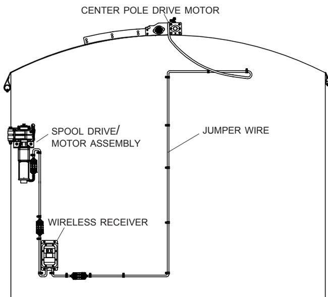
**STEP 8:** Route dual-conductor red (+) and black (-) wires to 24V power supply and connect in best way. Secure wire with wire clips and self-drilling screws.
