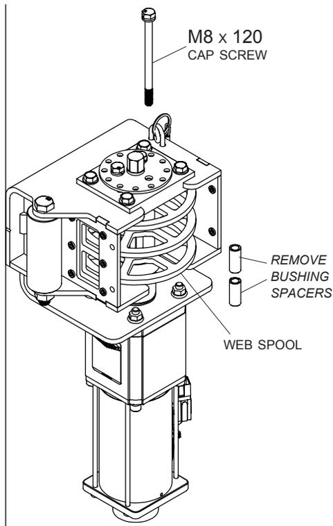
**STEP 9:** Route webbing through spool bracket web guide and insert bushing spacers into loops.
