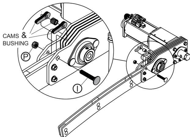
**STEP 3:** Install center pole drive motor. Insert key stock into center pole plug keyway. Align keyway on drive shaft by turning manual override shaft clockwise or counterclockwise and insert shaft into center pole plug.
