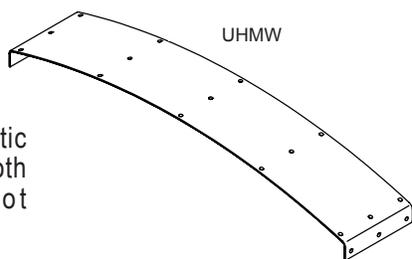
**STEP 2:** Install double support arch if required (not supplied).
