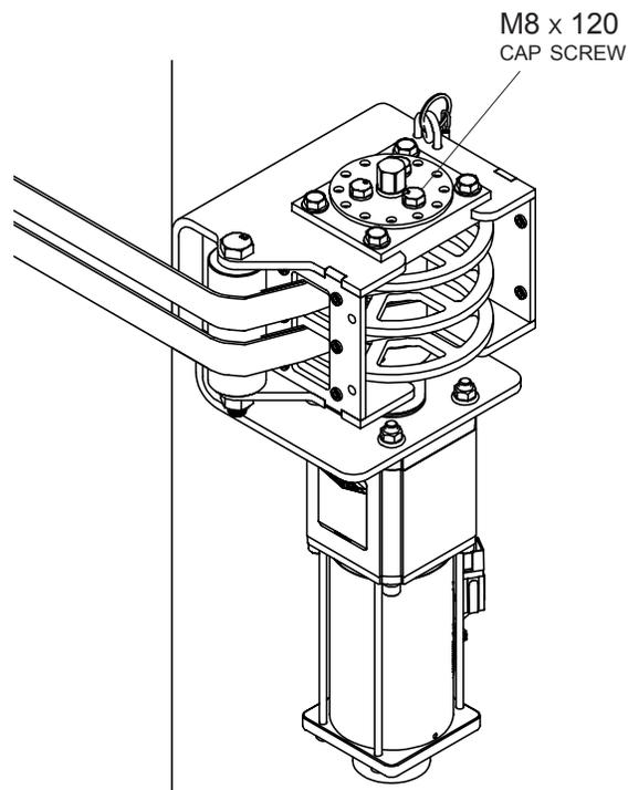
**STEP 11:** Rotate web spool until yellow screw **U** can be installed into holes on bottom of spool. Install screw and secure with nut **M**.
