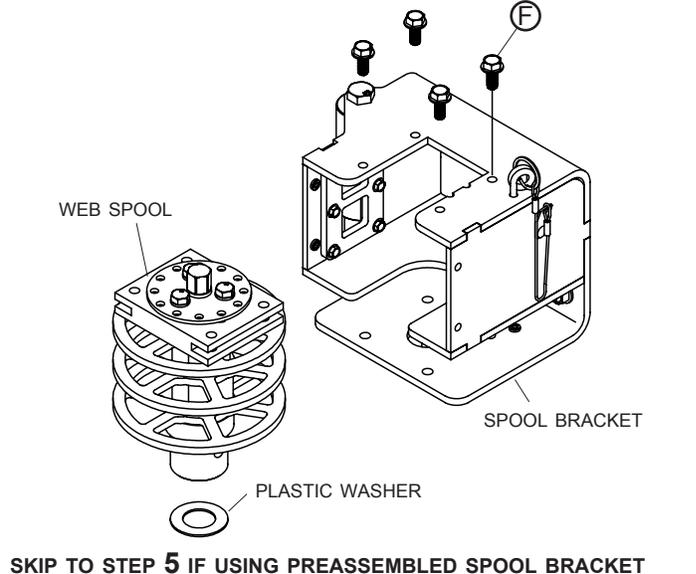
**STEP 3:** Fasten spool roller to spool bracket with M12 cap screw
