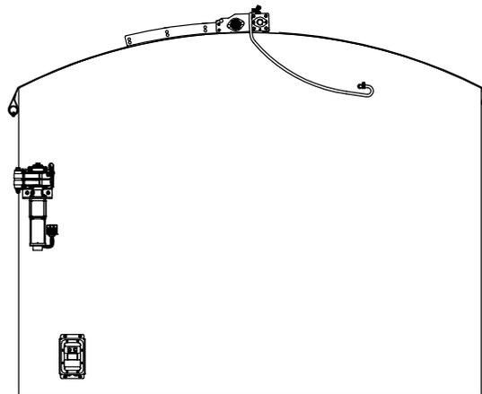
**STEP 19A:** Secure wire to motor gear with 1/2" wire clips and screws **B**, fastening through existing holes in motor.
