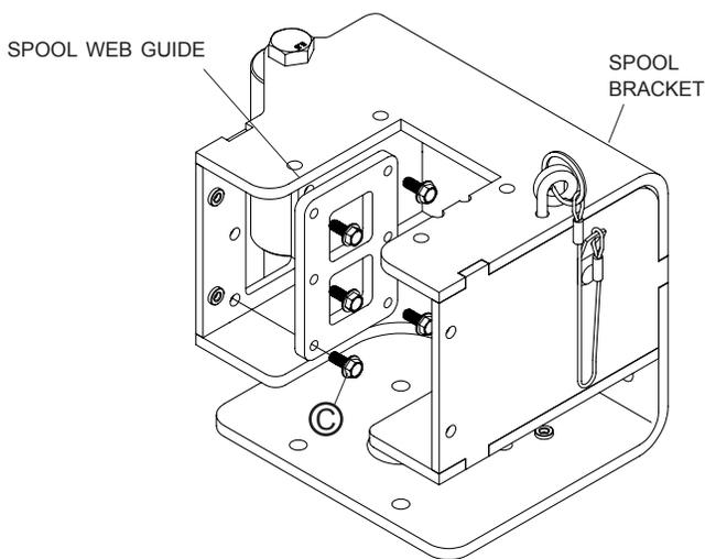
**STEP 5:** Determine location for spool bracket on front of box.
