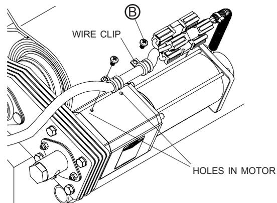
**STEP 20:** Route dual-conductor red (+) and black (-) wires to 24V power supply and connect in best way. Secure wire with wire-clips and self-drilling screws.
