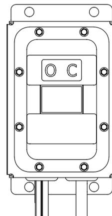
**STEP 11:** Measure as shown from top left 5mm hole. Mark and drill 51mm hole.
