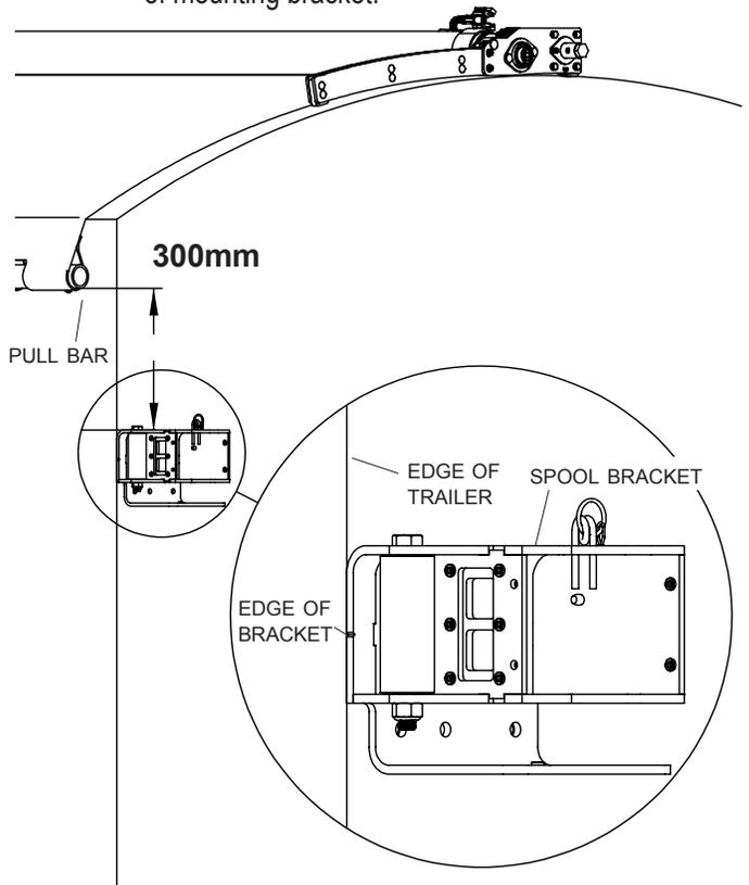
**STEP 5B:** Position top of bracket approximately 300mm below installed pull bar when in closed position.
