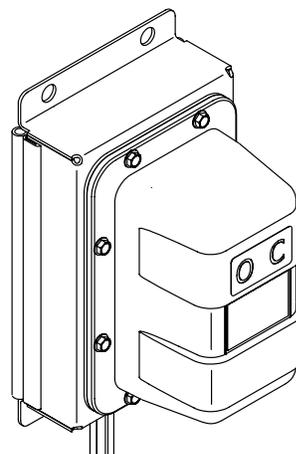
**STEP 10:** Using holes on receiver as guide, mark and drill four 5mm holes as shown.
