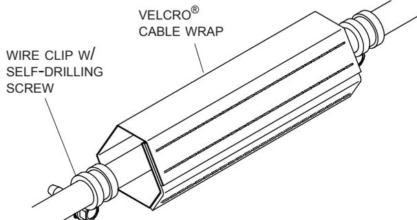
**STEP 18:** Route 3-conductor wire marked for spool motor through rubber grommet and to junction box on spool motor. Secure wire to bottom of spool bracket with wire clip and screw **D**. Secure wire to trailer with wire clips and self-drilling screws.
