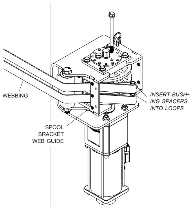
**STEP 10:** Push webbing and spacers back into spool and secure with M8 x 120 cap screw and lock washer. Tighten screws.
