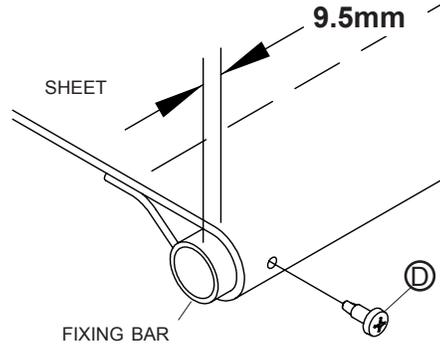
**STEP 10:** Place sheet on top of box with fixing bar hanging over right side of box. Move sheet forward or backward until center pole insert plug is 75mm from front face of hood.
