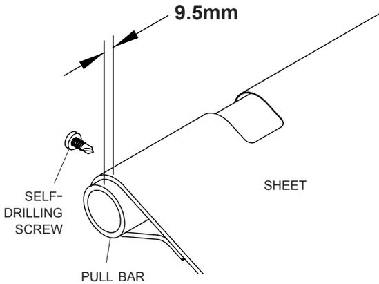
**STEP 9:** Repeat step 7 for fixing bar.
