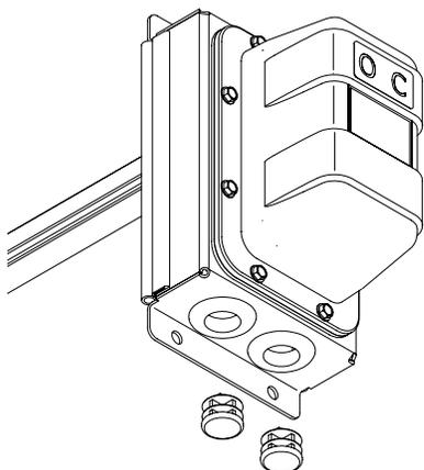
**STEP 13:** Install 1 1/2" rubber grommet into 81mm hole. Pass three wires through rubber grommet and align holes in bracket with drilled holes.
