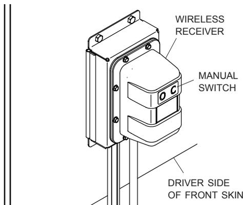
Verify wire lengths before drilling holes. Dual-conductor red (+) and black (-) wire must reach 24V DC power supply. Two marked 3-conductor wires must reach junction boxes on spool motor or center pole drive motor. Observe full motion of center pole motor and supply enough wire for motor to reach fully open and closed sheet positions.
