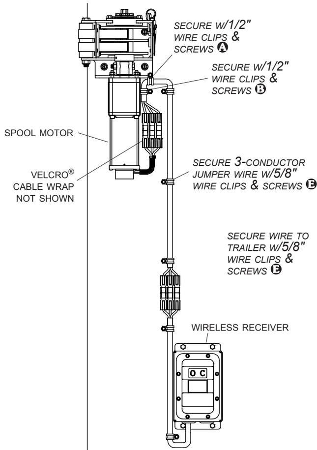
**STEP 6A:** Secure wire to motor with 1/2" wire clips and screws **(B)**, fastening through existing holes in motor assembly.
