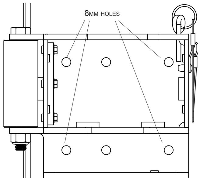
**STEP 5D:** Secure spool bracket to trailer with impact wrench and four self-tapping screws **J**.
