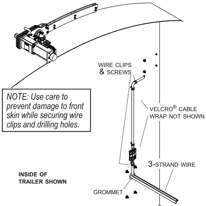
**STEP 19:** Repeat steps 15 to 16 for center pole drive motor, securing wire to box with wire clips and M6 screws.
