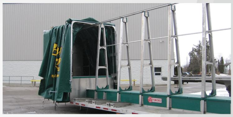
Glass-hauling systems are designed with a specialty all-aluminum headboard and unique monorail system that mounts on top of the A-frame and opens from the rear.
