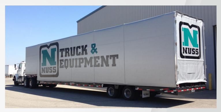
The ShurTite<sup>™</sup> system for drop-deck trailers is the only one in the industry that can clear either deck for maximum loading flexibility. Lower deck bows have a double set of wheels to transition to the top deck.
