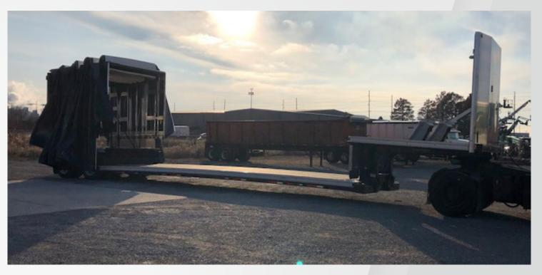
Lower deck bows come equipped with a triple set of wheels to transition to either front or rear raised decks. Drops must constitute a difference of 8 inches to completely transition system from front to rear.
